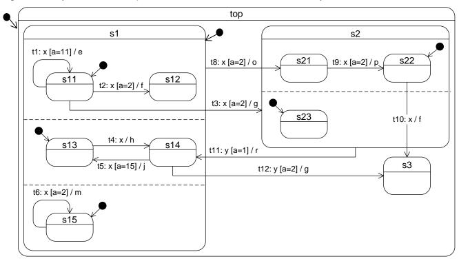
The current state of the statechart is the following state configuration: {top, s1, s11, s14, s15}. The value of variable a is 2. The incoming event is x.
