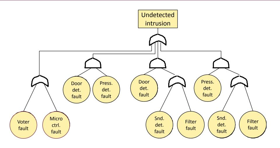
Single point of failure: Voter fault, microcontroller fault
