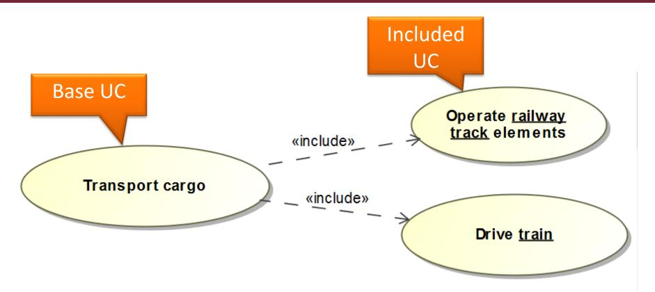
The included UC breaks down the complex core functionality into more elementary steps
