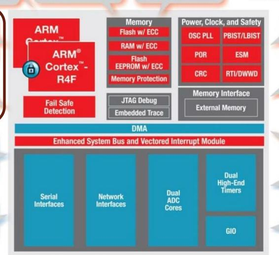
Memory BIST on all RAMs allows fast memory test at startup
