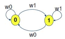
States in case of stuck-at 0/1 faults:
