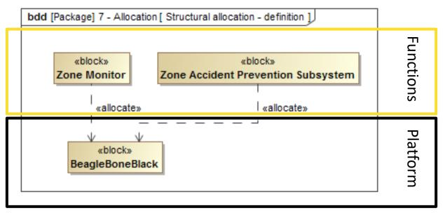
Wherever a BBB is used in the system, a zone monitor and an accident prevention subsystem is assumed to be allocated to it
