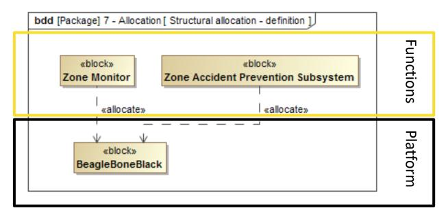
Wherever a BBB is used in the system, a zone monitor and an accident prevention subsystem is assumed to be allocated to it
