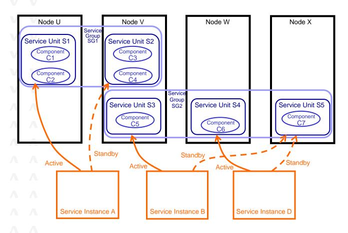
Service group SG1 supports a single service instance A, and service group SG2 supports two service instances B and D
