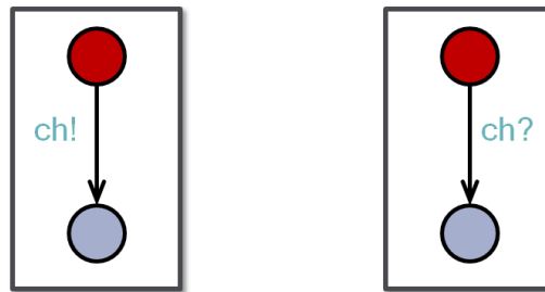
Figure 21. Simple synchronisation example
