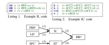
Fig. 2. Unified representation of Siemens PLC languages
