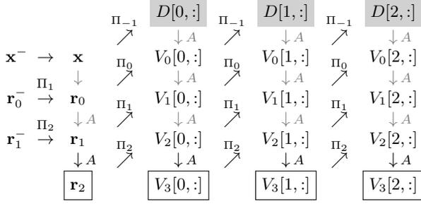
Fig. 3. Repetition step for IDR(s)STAB( $\ell$ ) extended for stochastic analysis with  $j = 2$  and  $s = 3$ . Quantities with a superscript  $-$  refer to the original values of the vectors before the repetition step.
