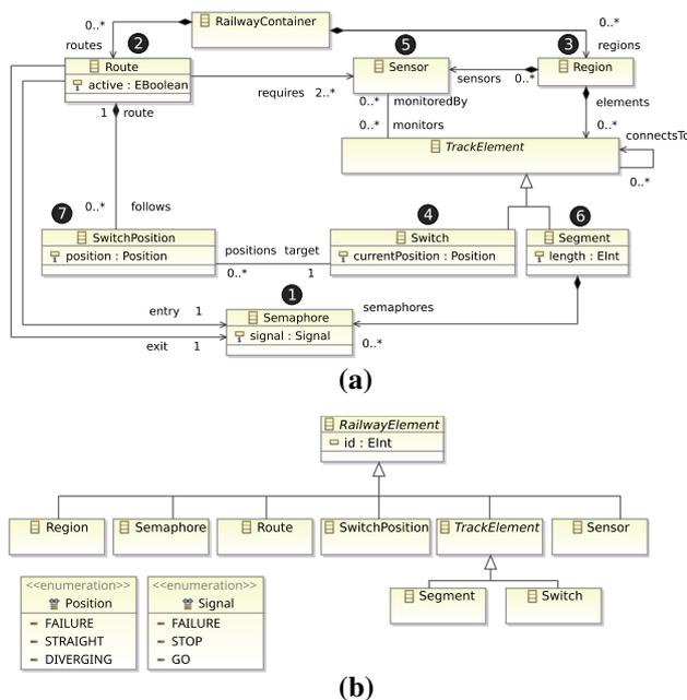
**Fig. 2** The metamodel of the Train Benchmark. **a** Containment hierarchy and references. **b** Supertype relations
