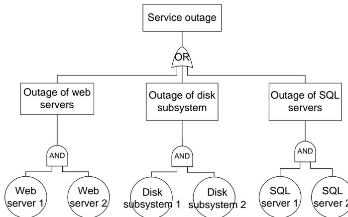
**Figure 6. Modified fault tree**
